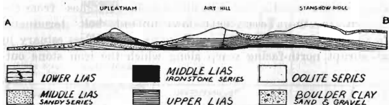
FIG. 5.—A cross-section from northwest to southeast across the Cleveland District to show the relations of the iron stone to the surface features and to the Geologic structure.
