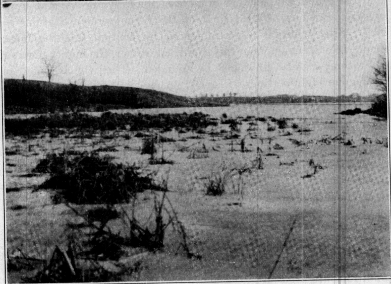
FIG. 5. ( Above ). Photo showing the confluence of the warm condenser water ditch (left) with a cold water ditch (right). Note also the ice sheet. The mixed water flows south, in the foreground of the picture. This represents Stations 7 (to the left in the "steaming" portion) and 7A to the right (in front of the ice).
