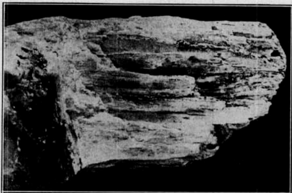
Fig. 2. Large zoisite crystal (white) bearing chalcopyrite (dark) on cleavage faces, Mary mine, Ducktown, Tenn.
