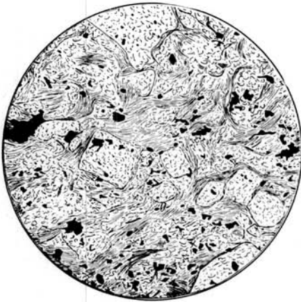
FIG. 2.—Sketch of microporphyritic felsite from dike in granite from H. O. Carr-Vedovell well, Lee County. Rectangular crystals represent altered feldspar; bundles of curving lines represent crystallites arranged in flowage pattern; black represents opaque minerals; and the rest is cryptocrystalline material. Magnification 120X.
