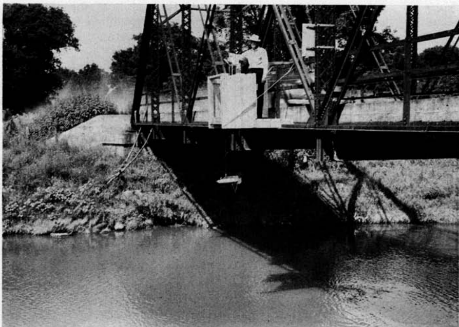
FIG. 2.—Testing the suspended sediment content of the Galena River. The study of stream transported sediment is very important in soil conservation and in deciding the efficiency of such engineering structures as dams, and irrigation ditches.
