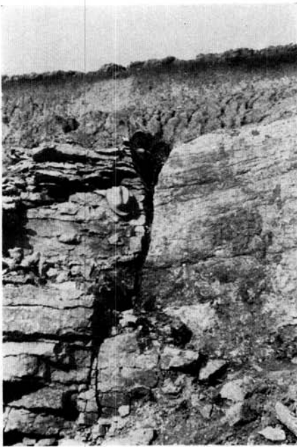
FIG. 3.—Filled joint at Site 1. Pick at contact of Champaign till above and plastic clay below.
