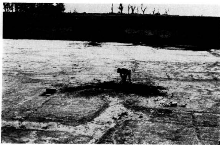
FIG. 2.—Filled joints and striations on stripped surface at Site 3.
