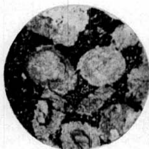
FIG. 6.—(Left) Thin section of Neda iron oxide spheroids in matrix of silty shale from Illinois (X18).
